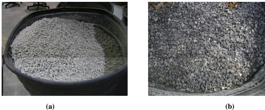
Figure 1 Aggregates; (a) Natural aggregate, (b) SS aggregate
