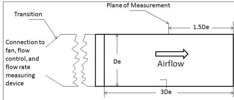
**Figure 1 Schematic for minimum length for pipe installation**
