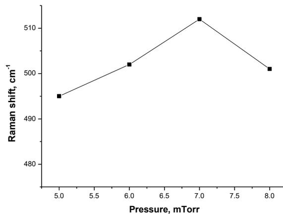
**Figure 3 Relationship Between Raman Shift and Sputtering Pressure**
