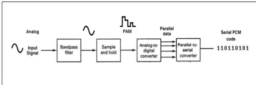
Figure 2.1 PCM transmitter of block diagram system.
